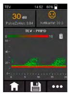
An indispensable function of the device is the phase pattern representation, so-called PRPD pattern. By means of this view, the user can clearly identify whether the measured data is due to partial discharges or simply noise – a big but decisive difference.
