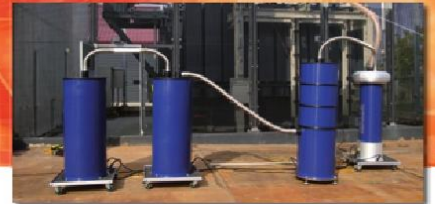
The DAC HV 250 allows testing up to 250 kV up to 500KV DAC
