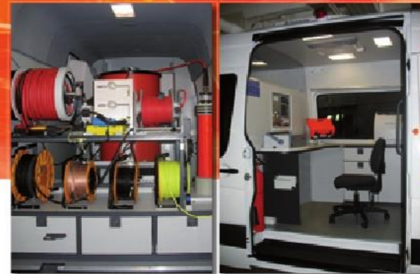
Test and diagnosis van with VLF CR-80 + OWTS M 60 and SPG 40
