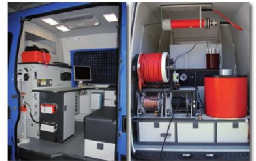
Test, diagnosis and fault location van Centrix 1-40 + VLF sine wave 54 + TanD + OWTS M 28
