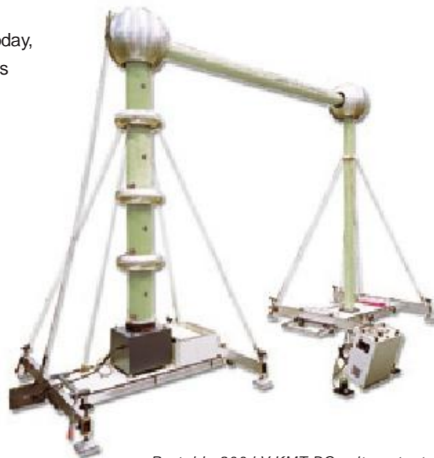
Portable 800 kV KMT DC voltage test system
